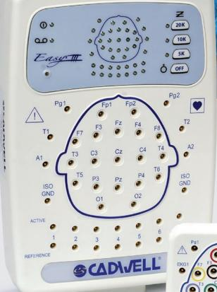
The 32 channel, 4 kHz, high-quality **Easy III** amplifier with integrated DC channels stays safely mounted to the wall or night stand. The color-coded **Remote Input Box** simplifies the connection of electrodes and sensors.
